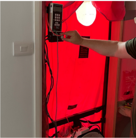
Air permeability 'blower door' test
